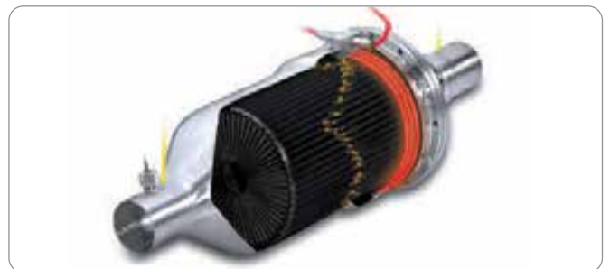
• Soot ignition following initial ignition
